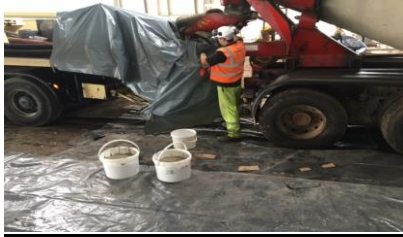
(1) 3 samples taken from flowing discharge – Start / middle / end
