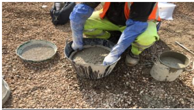
(4) Each sample is washed out by sieve and placed in sample bag
