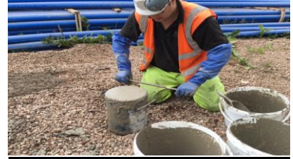
(3) Each sample measured in calibrated container
