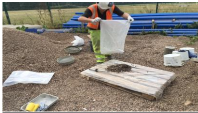
(5) Washed out sample is spread out on polythene sheet
