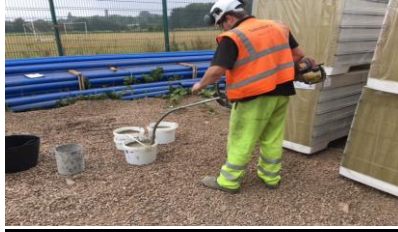
(2) Samples are vibrated with Twintec Poker
