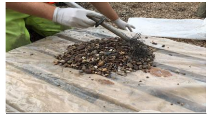
(6) Fibres are picked out by Magnet and placed in sample bag
